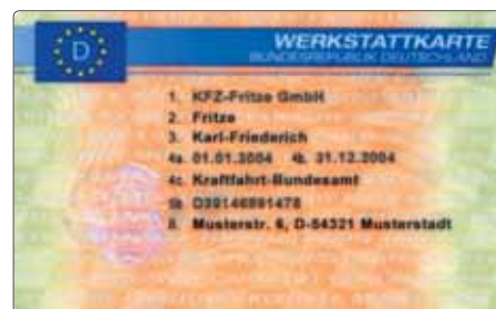
Workshop card: Identifies the authorised workshop, puts the digital tachograph in calibration mode and permits data to be output.
